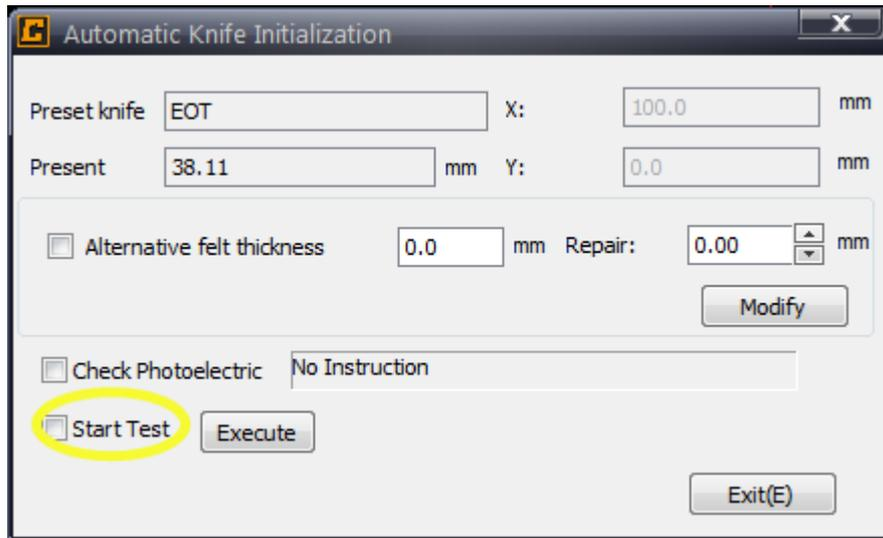
Before first use, select “start test”, then press any direction key, head will move to AKI device, after it done, check the position if it is correct.
